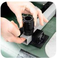
Place flat nut inside tube with one finger. Insert rail mount screw through pre-drilled hole in crosstube and into threaded hole in nut. Tighten by turning the mount.
