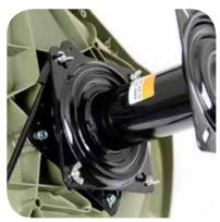
Hold pedestal against swivel. Insert hex head screws through swivel and pedestal slots. Thread wingnut onto screw. Do not tighten until all screws are in. Hold screw head with wrench, tighten wingnuts.
