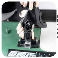
Push stem of rod holder into base. Listen for snap when seated. To remove, twist base and pull up on rod holder. Loosen large 3-arm knob to tilt.
