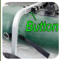
With wheel down, slide curved bar into frame until button pops up in hole.
