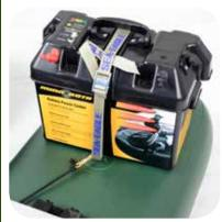
Run strap though one D-ring, over box, through second D-ring, back over box and through buckle. Pull tight and check strap frequently during
