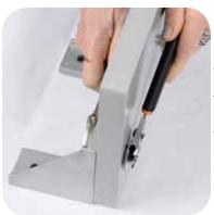
Insert bolts through bracket and though motor mount block. Apply washer and thread nut onto bolt. Tighten until bolt shows through nut and bracket is snug against block.
