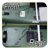
Hook clips on D-rings so that floor is pulled tight.
