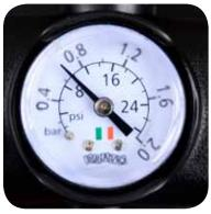
Working pressure is between 10 and 15 psi. Photo shows the minimum pressure of 10 psi.
