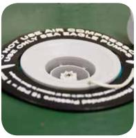
To deflate, push down on the valve stem and quarter turn it to the right. The stem will stay in the down position, allowing air to escape.
