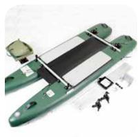
Slide seat/pedestal out of quick release. Remove aluminum board. Remove rod holders from their bases, bases can stay on the boat.
