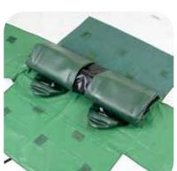
Keep folding and pushing air out to end of the pontoons.
