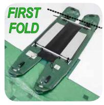
Place bag under front. Fold SUPCat toward the valves pushing air out as you go.
