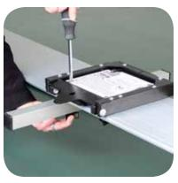
Align holes in the seat mount with holes in main board. Push screws down through Seat Mount and board. Long screws go in the rearward holes. Secure mount with knobs. Use screwdriver to hold screws heads.
