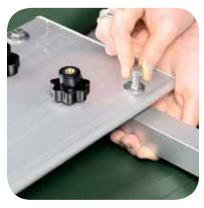
Place washers on the bolts. Push bolts through board. If holes do not align with crosstube, grip tube with fingers and push board with palm. Secure bolts with knobs. Hold bolt head with fingers or tool.
