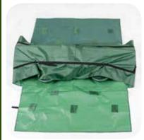
Fold side flaps over SUPCat in and secure with straps. Strap end goes through both loops and back through second loop.
